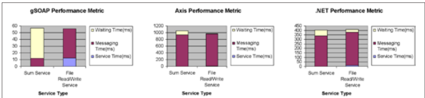
Figure 3: Performance analysis using gSOAP, .NET, and Axis Java
